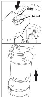
Lift out the bowl by the edges raising it the upper section and sliding it up the water spout. When it is high enough, rotate the bowl and spout until clear of the opening of the upper section.
